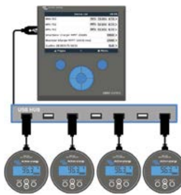
A maximum of four BMVs can be connected directly to a Color Control GX. Even more BMVs can be connected to a USB Hub for central monitoring.
